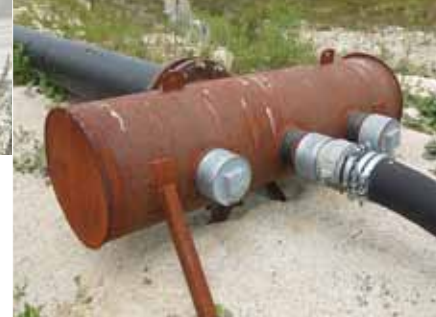
Dewatering Pipes and Manifold
