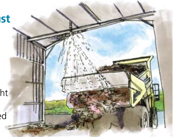
Use water sprays at drop points
